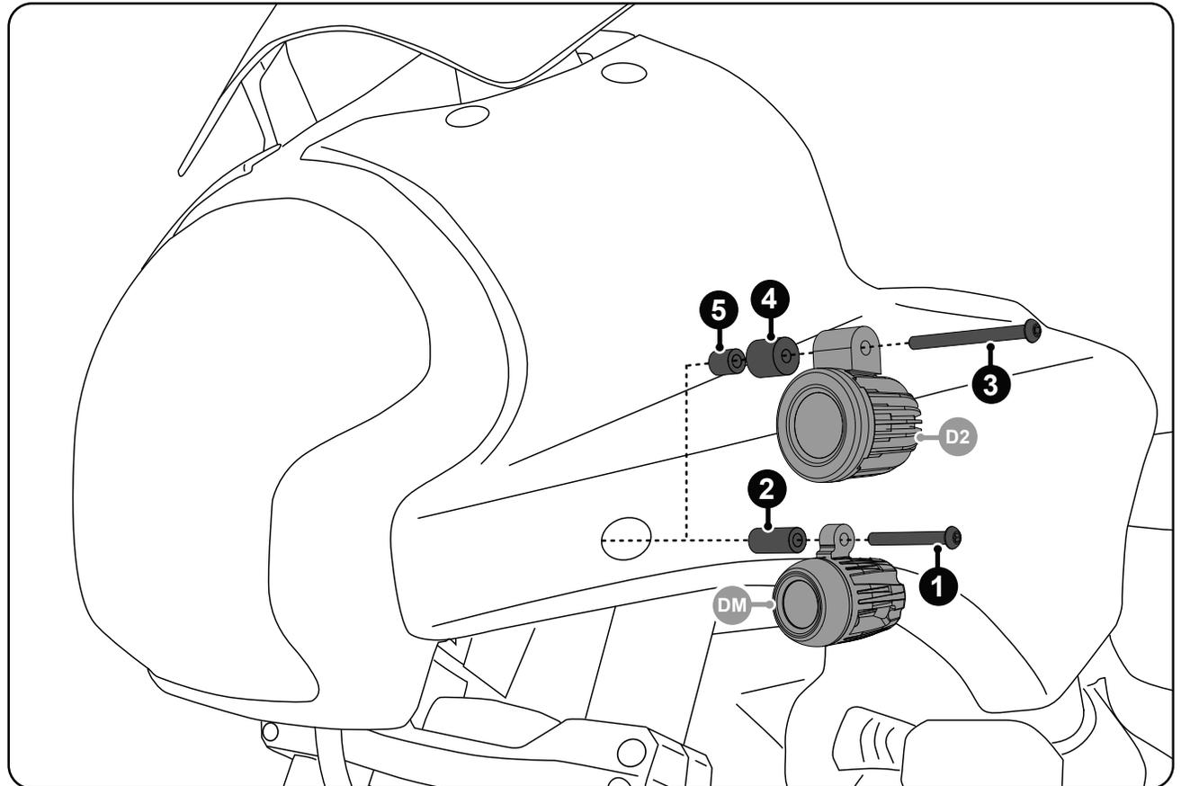
**Step One:** Remove the OEM screw from the mounting point illustrated on the upper fairing.
