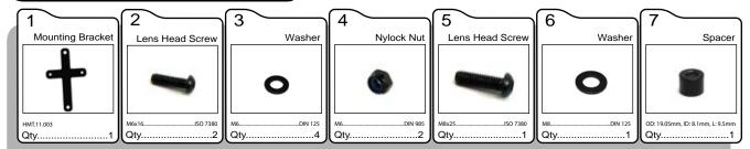
Step One: Remove the rectifier/regulator and horn/reflector assembly from their original locations. Use the M6 Bolts (#2), Washers (#3) and Nuts (#4) to mount the rectifier/regulator to the Mounting Bracket (#1). Next re-use the OEM hardware from the horn to bolt it to the Mounting Bracket (#1)
