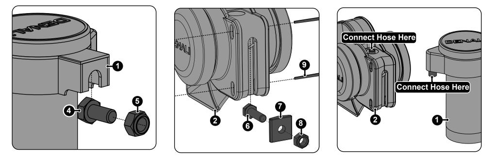
**Compressor Mounting:** Use the M8 bolt (#4) and nut (#5) to secure the compressor to you motorcycle.
